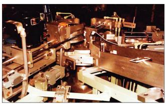
A large flux leakage and eddy current tester was designed and installed by MAC to inspect military ordnance such as shell bodies, shown above, using three seperate stations; a load station, a test station, and an accept/reject station. Two flux leakage tests were used for transverse and longitudinal defects, and eddy current tests for cracks and hardness included the Varimac® and the Production Comparator.
