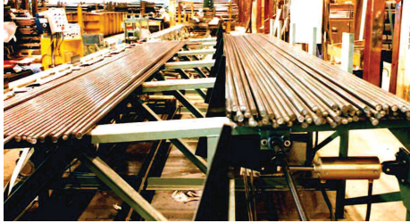
Intermediate Stop Arms hold back bars from a bundle that has just been broken out onto the Feed Rack in a bar mill.
