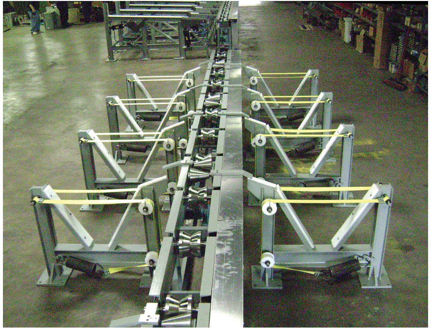
Outlet conveyor with accept/reject receiving pockets on either side for sorting. Feed racks are in the upper left. Test equipment will be installed between outlet conveyor and incoming Feed Racks. and Channel Roll Sections
