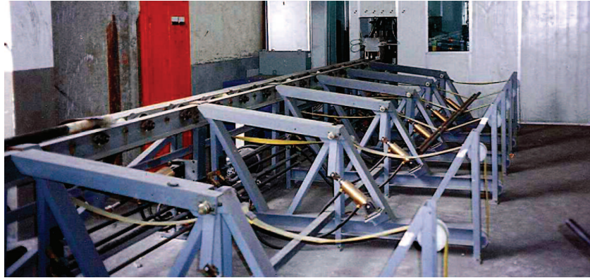
Exit channels and receiving pockets for a large feed system installed in a tube mill in China. Since both accept and reject pockets are located on the same side of the line, transfer arms are used. They are shown in the "down" position. Easy Down straps can be seen in the receiving pockets.
